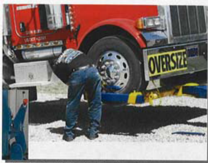
#8) Lift Zacklift fully into J-Lock. Pull strap over wheel and place hook into slot in rear of wheel tray.
