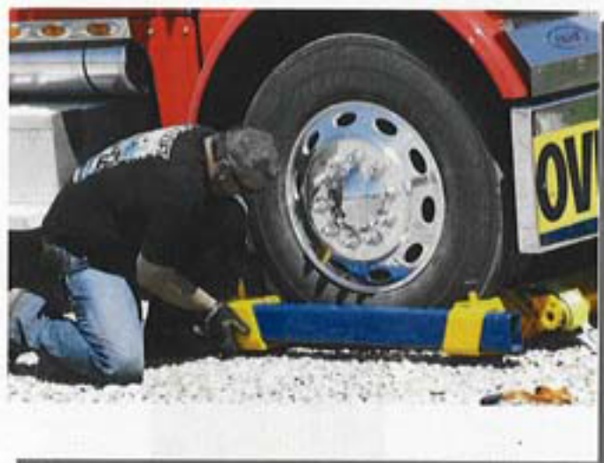
#7) Slide wheel tray onto wheel rod and against tire. Make sure pull pins are both fully engaged
