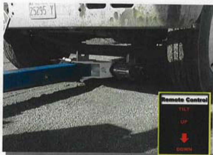
21) TILT down until tires touch the ground.
