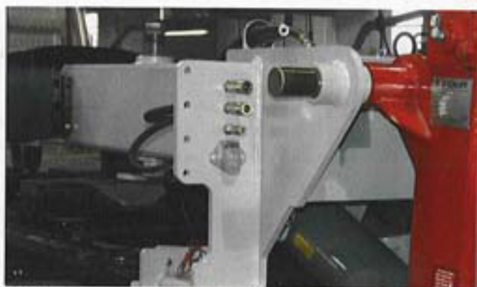
11. Be sure to use bushing (supplied) in Zacklift. Bolt securely.
