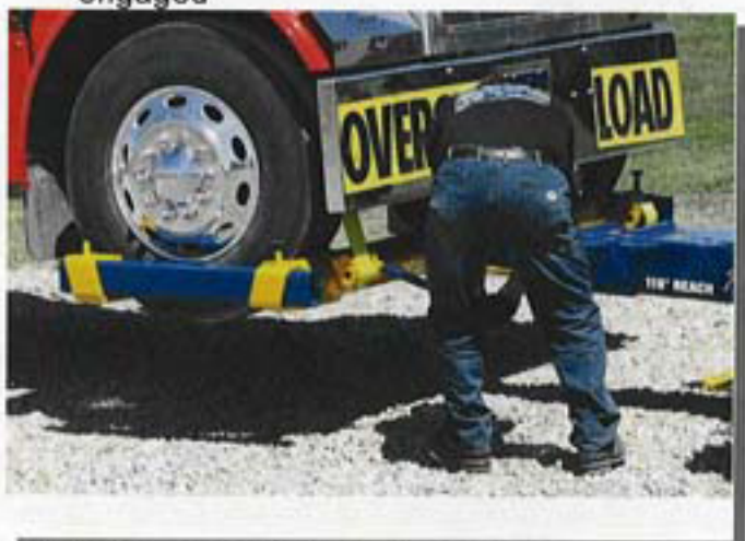
#9) Tighten strap with bar provided
