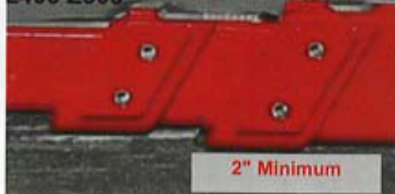
#11) Z403/Z303: Extend middle horizontal extend tube at least 2" from outer horizontal extend tube. This will create an equalization of pressure with inner tube, allowing head to pivot properly during towing. The head will appear to be locked against the inner extend tube but will disengage when turning.
